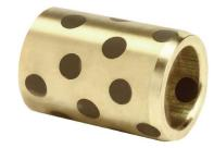
PCS Self-Lubricating Straight Bushings are solid bronze with graphite plugs. Nominal diameters ranging from 3/4" to 3" are available. PCS Self-Lubricating Straight Bushings reduce friction on leader pins and are press-fit into place. These bushings do not require grease which makes them great for food-grade, medical and high-speed applications.
